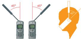
Once the antenna is correctly inserted and rotated, the Global Rental satellite phone will automatically search and connect to the Iridium network. When the phone connects to the network, the and a incons will show on the display.
